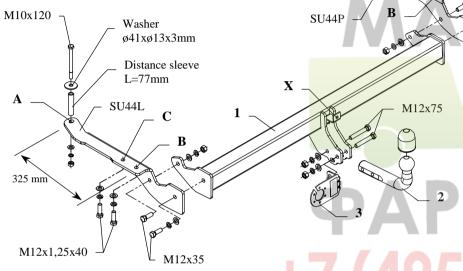
This towbar is designed to assembly in following cars: **SUBARU FORESTER, 5 doors,** produced since 1997 till 2000, catalogue no. **SU44** and is prepared to tow trailers max total weight **2000 kg** and max vertical load **75 kg**.
